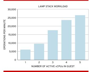
Scale-out of multiple virtual guests on a single host shows higher operations per minute than with bare metal on the same host—virtualization allows application performance scaling beyond the limitation of the bare metal application, providing better utilization of hardware resources.
