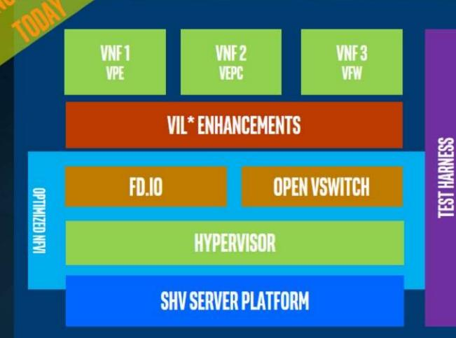
Develop Open Source *approximations* of Telco grade VNF's using optimized VNF + NFVi Infrastructure libraries, with Performance Characterization of *Sample* Traffic Flows using open source Test Harness
