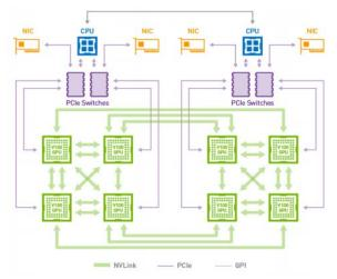
Figure 4: Hybrid Cube Mesh NVLink Topology Source: NVIDIA website
