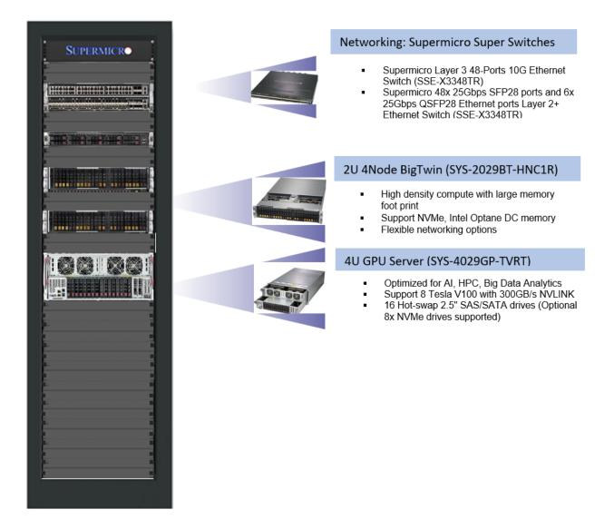
Figure 1: Hardware components of the stack which ran the MLPerf Training v0.6 benchmark described in this white paper.
