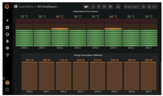
Figure 12: Monitoring GPU temperature and power usage
