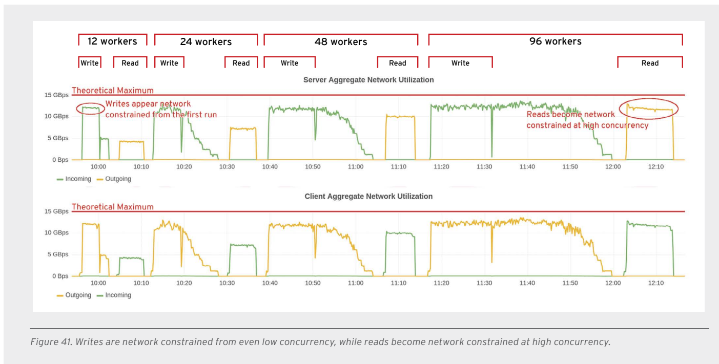
Figure 41 shows network activity for both writes and reads for increasing levels of concurrency.
