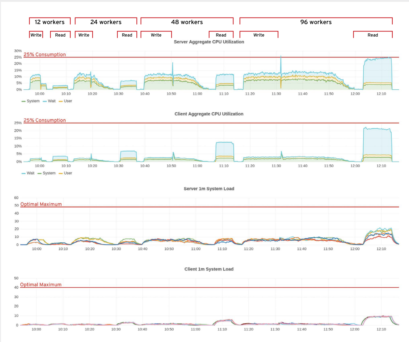
Figure 42. Server and client CPU and system load for 128GB files on a distributed-replicated volume on RAID 6 bricks.
