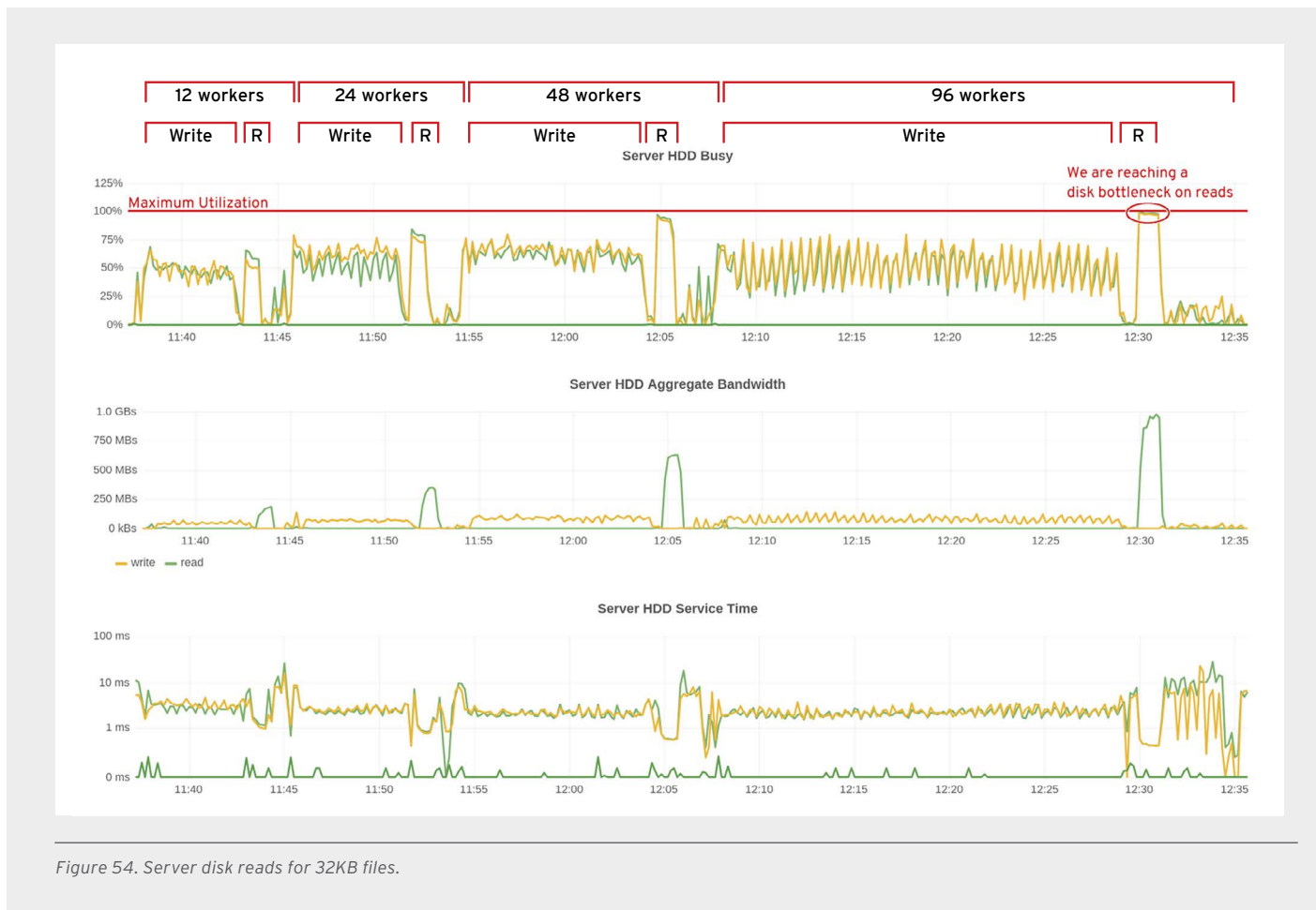
Figure 54 illustrates that a potential bottleneck is being approached on server disk reads as concurrency is increased to 96 workers.
