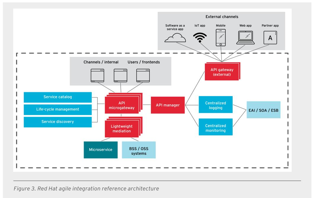
Figure 3. Red Hat agile integration reference architecture
