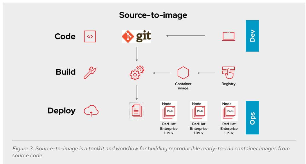
Red Hat OpenShift image streams can be used to watch changes to external images deployed in your cluster. Image streams work with all the native resources available in Red Hat OpenShift, such as builds or deployments, jobs, replication controllers, or replica sets. By watching an image stream, builds and deployments can receive notifications when new images are added or modified and react by automatically launching a build or deployment, respectively.
