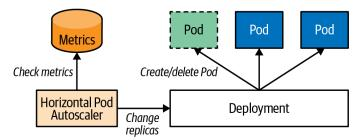
Figure 29-1. Horizontal Pod autoscaling mechanism
