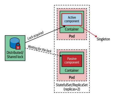
Figure 10-2. In-application locking mechanism
