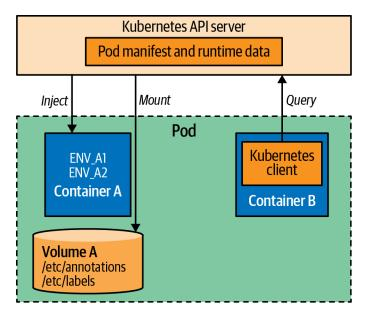
Figure 14-1. Application introspection mechanisms
