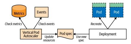
Figure 29-4. Vertical Pod autoscaling mechanism
