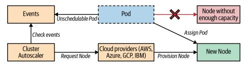
Figure 29-5. Cluster autoscaling mechanism
