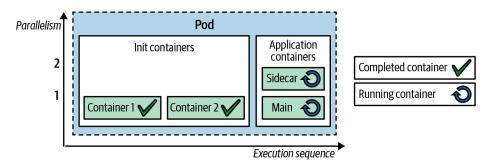
Figure 15-1. Init and application containers in a Pod
