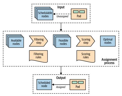
Figure 6-1. A Pod-to-node assignment process
