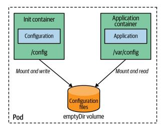
Figure 21-2. Immutable configuration with an init container
