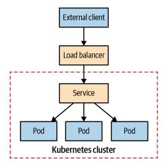
Figure 13-6. Load balancer service discovery
