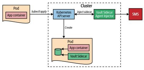
Figure 25-5. Vault Injector
