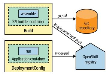
Figure 30-3. S2I build with Git source as input
