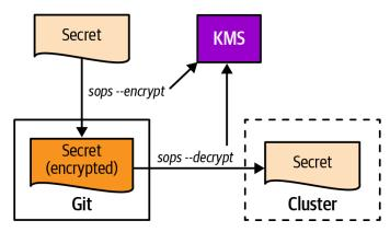
Figure 25-3 illustrates how sops handles encryption and decryption on the client side.
