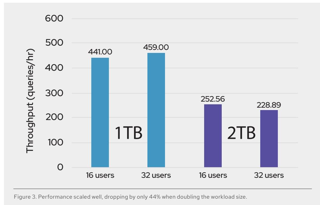
During testing, the cluster was instrumented to understand utilization and scalability. Results were then compared to other cloud-based configurations for Db2.
