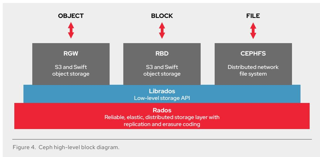
From an architectural perspective, Ceph provides software modules that are designed for different tasks and responsibilities, including:
