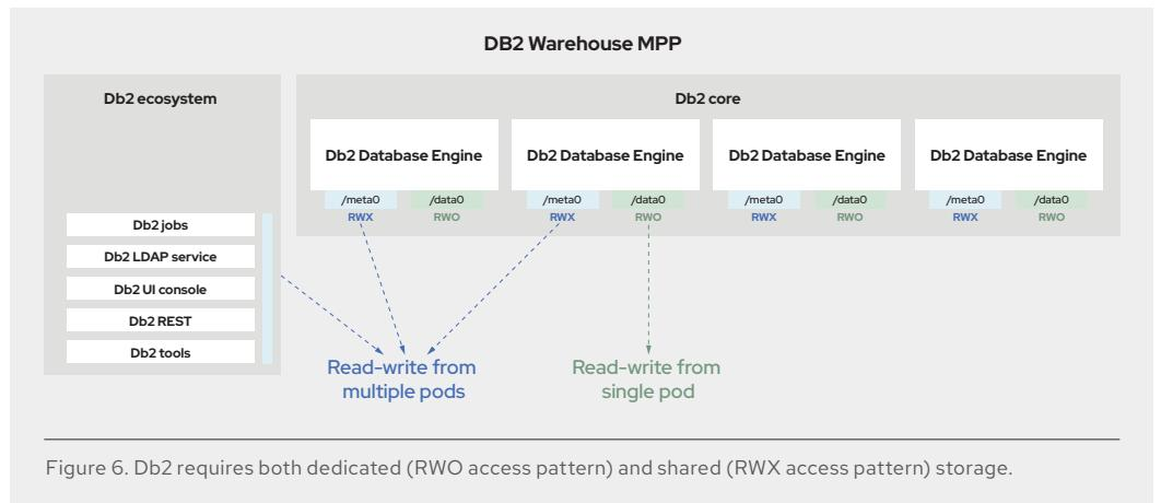
With Red Hat OpenShift Container Storage, both the type of storage (e.g., file or block) and the storage technology itself (e.g., cloud-based storage volumes or direct-attached storage) can be configured appropriately to match workload needs.
