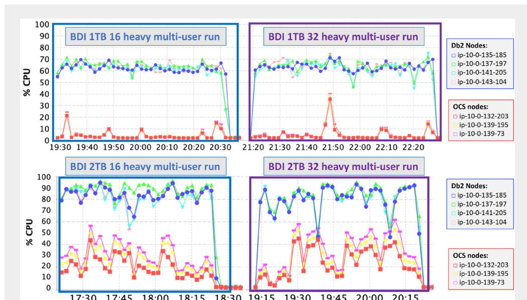
Figure 7. NMONVisualizer output for the 16 and 32 heavy multi-user runs showing system utilization for each node.
