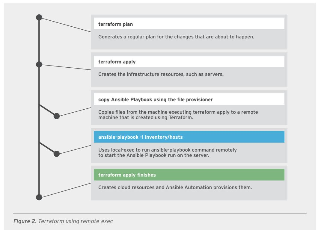
This approach works well when Terraform is responsible for creating the resources, and Ansible Automation is installed and invoked on the remote machine.
