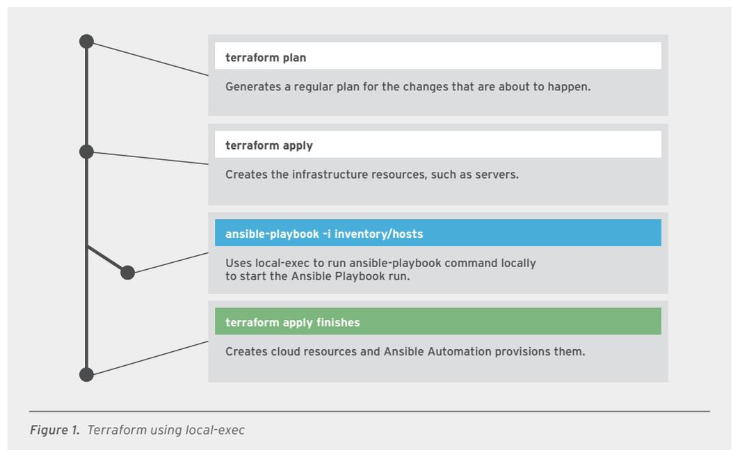
This approach works well when Terraform is responsible for creating resources and Ansible Automation is installed on the same machine with access to the newly created resources—i.e., Terraform and Ansible Automation are both installed on the same control node used to execute resource creation commands, like a bastion host or management proxy.
