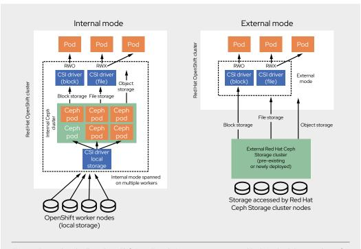
Figure 1. External mode allows OpenShift Data Foundation to access an external Red Hat Ceph Storage cluster for block, file, or object storage.
