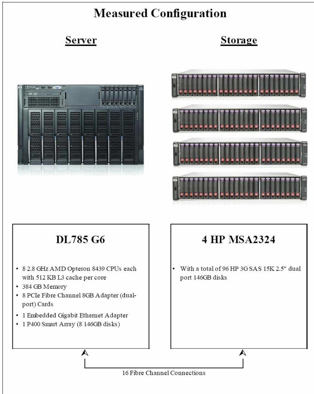
*Figure 4: Hardware Configuration*
